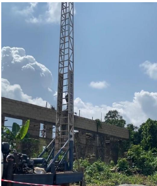
FIG 1.1 DRILLING MACHINE USED TO DRILL 350 FT BELOW GROUND LEVEL
